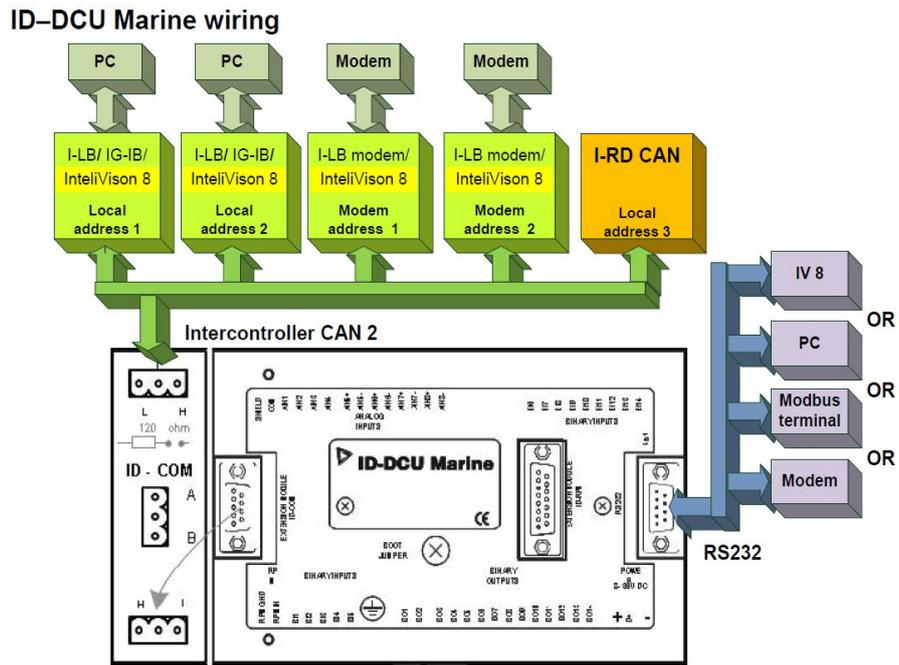
Image 9.6 IntelliDrive – DCU Marine wiring
