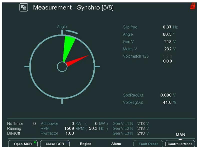
Image 4.10 Synchroscope screen
