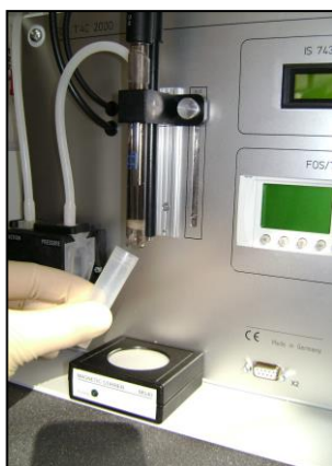
Removing the protective cap
