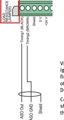
Via the auxiliary synchronization output (ASO), the ignition controller sends the ignition impulse of the first cylinder in firing order to the DetCon2/20. All other ignition timing points are calculated by the DetCon2/20.
