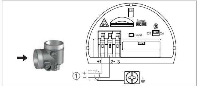
Fig. 25: Compartiment de raccordement - Module radio PLICSMOBILE 81
