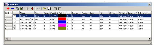
Shows name, dimension, appropriate controller, communication object, color etc. of selected channels.
