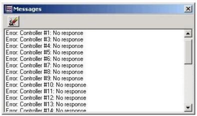
Shows error messages while WinScope is trying to connect to the controller or read the configuration from the controllers.
