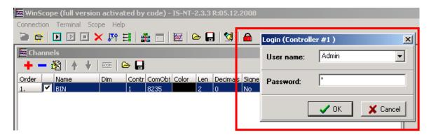
In Controllers window doubleclick on the controller that you want to connect to. For IG/IS-NT controllers user has to be selected prior to password entering. Level of entered password is marked in the lock sign.
