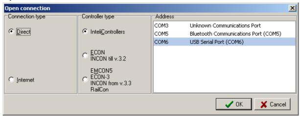
Controller type  $\rightarrow$  select connection to InteliController, ECON/INCON or EMCON5/RailCon controller. Address  $\rightarrow$  select to which communication port of the PC the controller is connected
