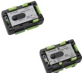
This portion of Installation instructions is dedicated to controllers with High-Side Low-Side Switch. These controllers include: IG-NT-BB, IG-NTC-BB, IS-NTC-BB, IM-NT-BB and IM-NTC-BB
