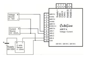
Note: Unused inputs must be connected to COM and the corresponding DIP switch must be OFF.
