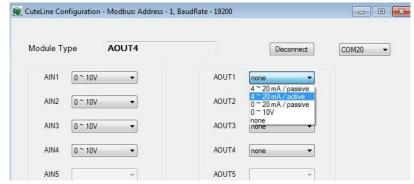
Launch the software and click on "Connect". Select the input/output type which is required on the individual input/output and click on "Ok". If the configuration is successful, you will receive a pop up box message to notify you about it. After this is completed, click on "Disconnect" and turn off the power supply to the module. This completes the sensor type configuration process.
