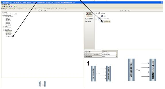
Sensors that can be configured in GenConfig that supports this module include 0-10V, 0-20mA and 4-20mA.
