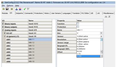
Note: CuteLine AOUT4 module supports only the first four inputs(AIN1 to AIN4) to each of the generic extension module added.
