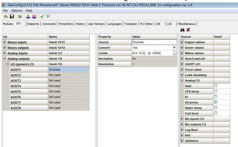
Note: CuteLine AOUT4 module supports only the first four outputs(AOUT1 to AOUT4) to each of the generic extension module added.
