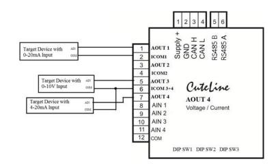
With DIP SW1(DIP SW1:1 to SW1:4), the type of output(OFF→Current, ON→Voltage) is selected. Each of the 4 poles of DIP SW1 is assigned to the corresponding input. If the sensors are connected according to the picture shown on the right, DIP SW1 must be configured as:
