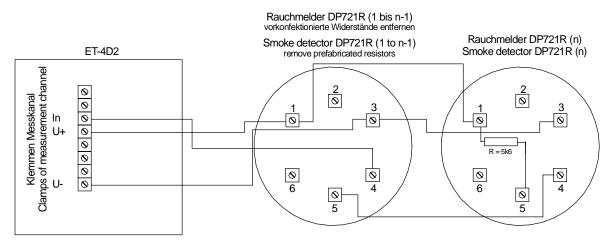
In all smoke detectors resistors (R = 5.6 k $\Omega$ ) have to be installed according to the figures. The resistors are included in the red protection caps or already installed.
