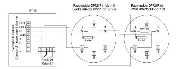
Inside the ET-8D Relay K21 has to be included into wiring. For several smoke detector lines the supplies (clamp 1) should all be done from the mid contact ("Common") of Relay K21. In all smoke detectors resistors (R = 5.6 k $\Omega$ ) have to be installed between clamps 1 and 5. For the last smoke detector of each line and additional terminating resistor (R<sub>ab</sub> = 5.6 k $\Omega$ ) has to be installed additionally between clamps 1 and 6.
