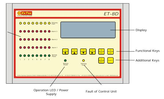
The display indication and the assignment of the functional keys F1 to F6 varies in the different operation modes of the ET-8D. The corresponding assignment of the functional keys is indicated in the line at the bottom of the graphic display.
