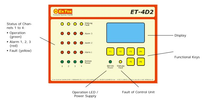
The display indication and the assignment of the functional keys F1 to F6 varies in the different operation modes of the ET-4D2. The corresponding assignment of the functional keys is indicated in the two lines at the bottom of the graphic display.
